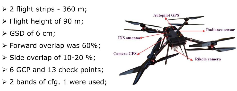
$\succ$  GPS time for each event of cube acquisition (first band); > Acquisition time of the remaining bands were estimated by the nominal time differences (22 ms);  $\succ$  Double frequency GNSS receiver grabbed raw data - 1 Hz;
