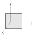
b) Imagine a charge q at the center of a cube of edge length 2L. Then:  $\Phi=q/\varepsilon_0$ . Here the square is one 24th of the surface area of the imaginary cube, so it intercepts 1/24 of the flux. That is,  $\Phi=q/24\varepsilon_0$ .
