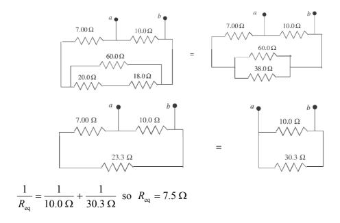
**26.56:** Recognize that the ohmmeter measures the equivalent parallel resistance, not just X.
