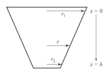
$$dR = \frac{\rho L}{A} = \frac{\rho dx}{\pi r^2} \text{ where } r = r_1 - \left(\frac{r_1 - r_2}{h}\right) x.$$
