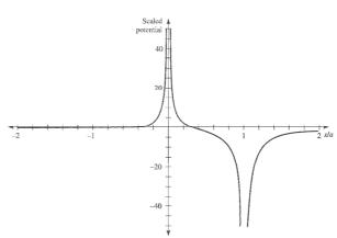
e) For x >> a:  $V \approx \frac{-kqx}{x^2} = \frac{-kq}{x}$ , which is the same as the potential of a point charge -q. (Note: The two charges must be added with the correct sign.)
