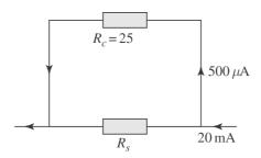
b) For a 500-m voltmeter, the resistances are in series:
