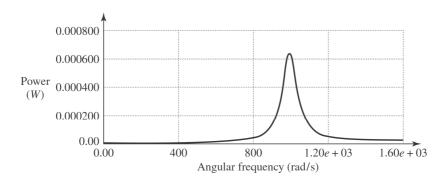
Note that as the angular frequency goes to zero, the power and current are zero, just as they are when the angular frequency goes to infinity. This graph exhibits the same strongly peaked nature as the light red curve in Fig. (31.15).
