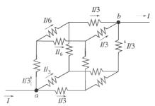
Let current I enter at a and exit at b. At a there are three equivalent branches, so current is I/3 in each. At the next junction point there are two equivalent branches so each gets current I/6. Then at b there are three equivalent branches with current I/3 in each. The voltage drop from a to b then is  $V = \left(\frac{I}{3}\right)R + \left(\frac{I}{6}\right)R + \left(\frac{I}{3}\right)R = \frac{5}{6}IR$ .
