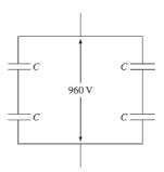
$C_{\rm eq} = \frac{C}{2} + \frac{C}{2} = C$ . So the total capacitance is the same as each individual capacitor, and the voltage is spilt over each so that  $V = 480\,$  V. Another solution is two capacitors in parallel that are in series with two others in parallel.
