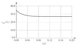
**30.72:** a) Immediately after  $S_2$  is closed, the inductor maintains the current i = 0.180 A through R. The Kirchoff's Rules around the outside of the circuit yield:
