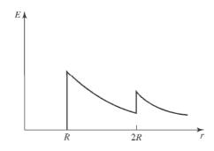
**22.38:** a) r < a,  $E = \frac{1}{4\pi c_0} \frac{Q}{r^2}$ , since the charge enclosed is Q.
