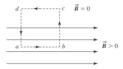
**28.79:** a) Below the sheet, all the magnetic field contributions from different wires add up to produce a magnetic field that points in the positive x-direction. (Components in the z-direction cancel.) Using Ampere's Law, where we use the fact that the field is antisymmetrical above and below the current sheet, and that the legs of the path perpendicular provide nothing to the integral: So, at a distance a beneath the sheet the magnetic field is:
