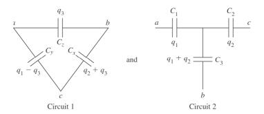
From Circuit 1:  $V_{ac} = \frac{q_1 - q_3}{C_v}$  and  $V_{bc} = \frac{q_2 + q_3}{C_x}$ , where  $q_3$  is derived from  $V_{ab}$ :
