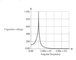
d) When the angular frequency is zero, the inductor has zero voltage while the capacitor has voltage of 100 V (equal to the total source voltage). At very high frequencies, the capacitor voltage goes to zero, while the inductor's voltage goes to 100
