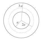
Apply Ampere's law to a circular path of radius 2a.  $B(2\pi r) = \mu_0 I_{\text{encl}}$
