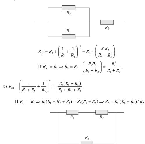
**26.49**: a) We wanted a total resistance of 400  $\Omega$  and power of 2.4 W from a combination of individual resistors of 400  $\Omega$  and 1.2 W power-rating.
