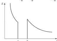
b) (i) Inner charge per unit length is  $-\alpha$ . (ii) Outer charge per length is  $+2\alpha$ .
