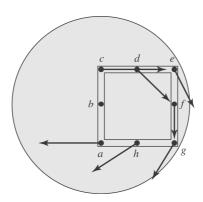
b) The induced emf on the side ac is zero, because the electric field is always perpendicular to the line ac.
