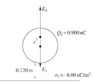
The electric field  $\vec{E}_1$  of the sheet of charge is toward the sheet, so the electric field  $\vec{E}_2$  of the sphere must be away from the sheet. This is true above the center of the sphere. Let r be the distance above the center of the sphere for the point where the electric field is zero.
