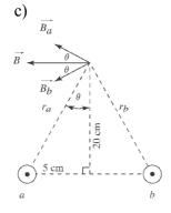
Note that  $\vec{\boldsymbol{B}}_a \perp r_a$  and  $\vec{\boldsymbol{B}}_b \perp r_b$
