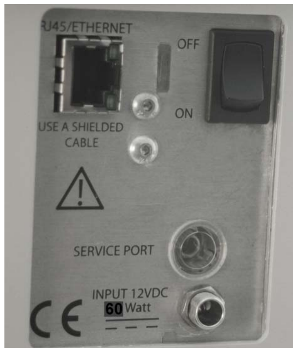
Figure -2 ASD Spectrometer back panel showing Ethernet connection, power switch, and power input jack.
