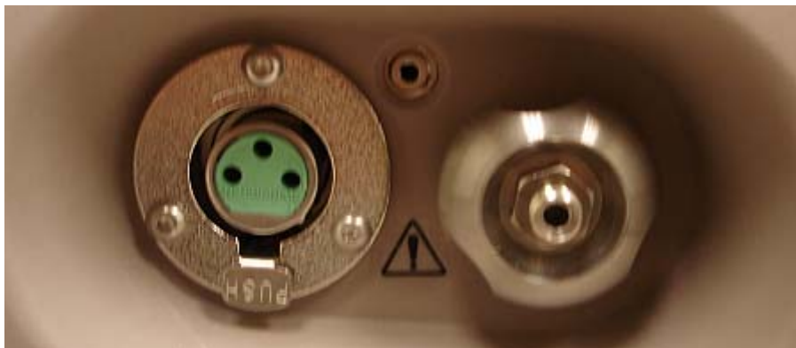
Figure -3 Enhanced view of the front panel with the fiber cable connector and accessory power jack for probe for the AgriSpec, LabSpec, and TerraSpec.
